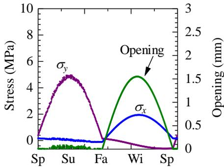
(a) Stresses at the fracture tip and fracture opening and closure with time.
