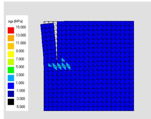
(c) Fracture opening/deformation and  $\sigma_x$  distribution in winter.
