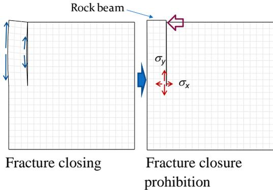
(a) Fracture closure prohibition and the stress development at the fracture tip.
