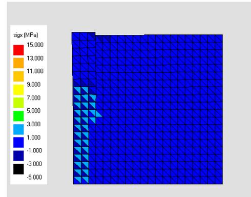
(b) Fracture closure/deformation and  $\sigma_x$  distribution in summer.
