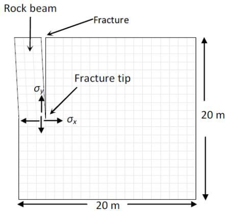
Fig. 1. Model showing rock mass (20 m x 20 m) with 10 m rock beam.
