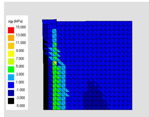
(c) Fracture opening/deformation and  $\sigma_y$  distribution in winter.
