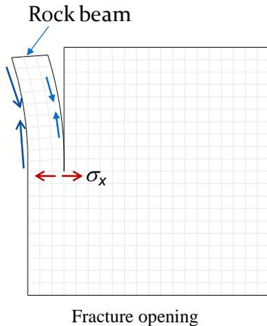
(b) Fracture opening due to the shrinkage difference.
