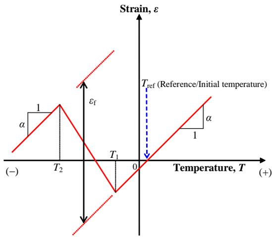
Fig. 4. Model for expansion due to freezing of pore water.
