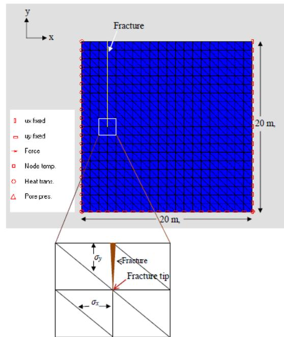
Fig. 2. Finite elements mesh configuration and Element where stress values are examined.
