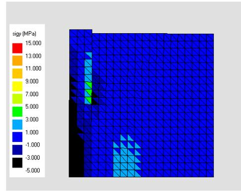
(b) Fracture closure/deformation and  $\sigma_y$  distribution in summer.
