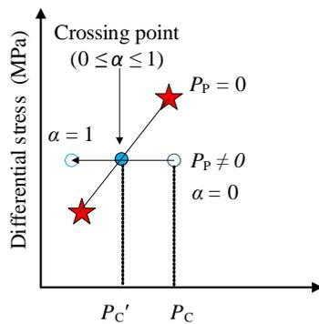
Fig. 1 Evaluation of  $\alpha$  by the modified failure envelope method
