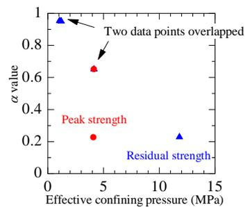
Fig. 3 Biot's constant variation with effective confining pressure for Shikotsu welded tuff
