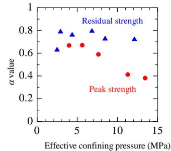
Fig. 2 Biot's constant variation with effective confining pressure for Kimachi sandstone
