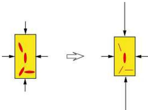
Fig. 10. Permeability decreased before peak stress due to closure of microcracks which are not parallel to the loading axis.
