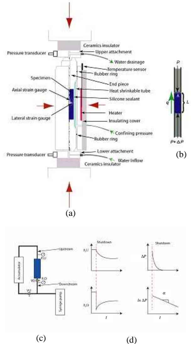
Fig. 2. Experimental setup. (a) Ultra compact triaxial cell and accessories for constant flow method (b) Basis for permeability measurement in constant flow method. (c) Schematic diagram for transient pulse method (d)  $\alpha$ - gradient of time-ln  $\Delta P$  in transient pulse method.
