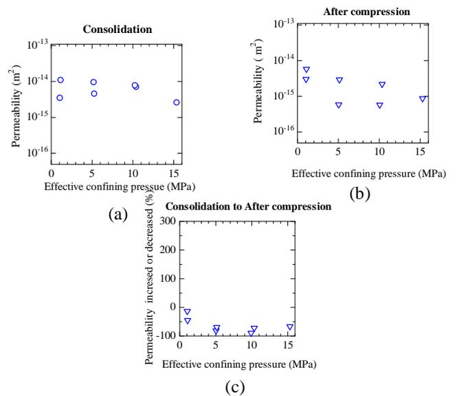
Fig. 5. Permeability after consolidation (a), after compression (b) and its changes (c) of Shikotsu welded tuff.
