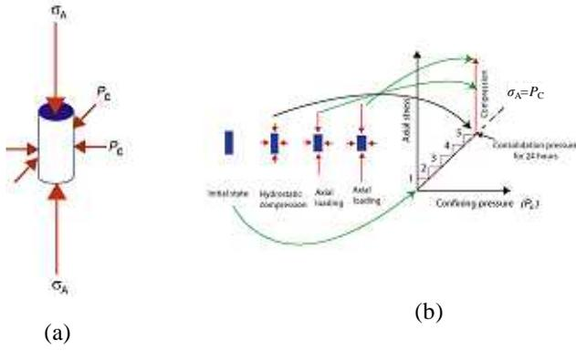
Fig. 3. The triaxial test and the experimental procedure. (a) The triaxial test (b) Procedure to reach the target consolidation pressure and compression.
