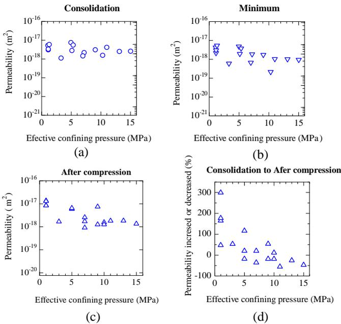
Fig. 7. Permeability after consolidation (a), at minimum (b), after compression (c) and it's changes (d) of Kimachi sandstone.
