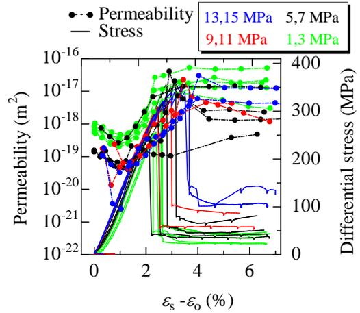
Fig. 8. Stress and permeability relation of Inada granite
