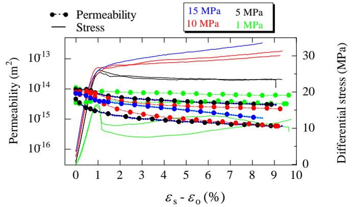
Fig. 4. Stress and permeability relation of Shikotsu welded tuff.
