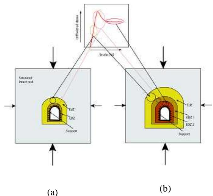
Fig. 1. EdZ and EDZ around an excavation. (a) Initial state (b) Final (residual strength) state.
