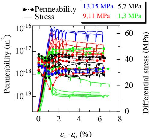
Fig. 6. Stress and permeability relation of Kimachi sandstone.
